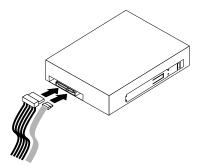
Figure 20. Connecting the optical drive
